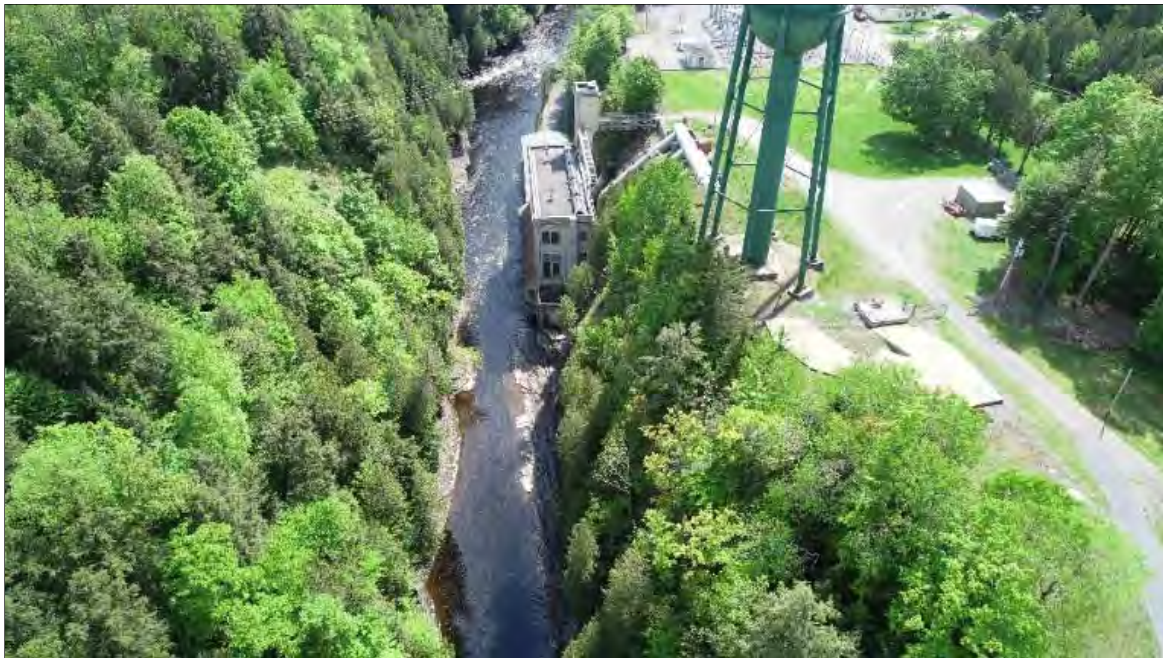
PHOTO 8 LOWER PORTION OF TRENTON BYPASS REACH, SHOWING POOL BACKWATERED BY TAILRACE
